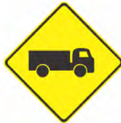
FIGURE 6.2 Typical W5-22 sign face (TfNSW)
